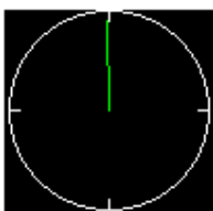
(b) The display with a normal psk31 signal. The vector flips between 0 and 6 o'clock
