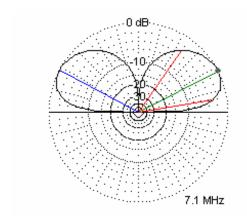
Radiation pattern of a Vertically Oriented Buddipole™ on 7.1 MHz with a center height of 10 feet.
