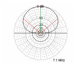
Radiation Pattern of a Horizontal Buddipole™ on 7.1MHz with a center height 10 feet and a resulting take-off angle of 90 degrees.
