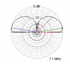
Radiation pattern of a Vertically Oriented Buddipole™ on 7.1 MHz with a center height of 10 feet over salt water.
