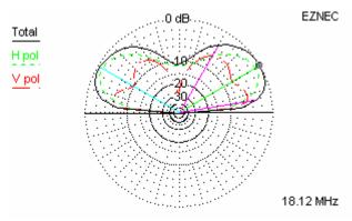
Radiation pattern of an L configuration Buddipole™ on 18.12 MHz with a center height of 25 feet.
