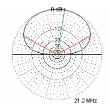
Radiation Pattern of a Horizontal Buddipole<sup>TM</sup> on 21.2 MHz with a center height 10 feet and a resulting take-off angle of 80 degrees.
