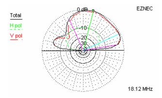
Radiation pattern of an L oriented Buddipole™ on 18.12 MHz with a center height of 10 feet.
