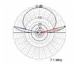
Radiation pattern of a Horizontal Buddipole™ on 7.1 MHz with a center height of 10 feet at the crest of a hill with the earth sloping away in all directions.
