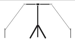
Set the Buddipole up as you normally would. The RED COIL goes on the left, or hot side of the coax and the BLACK coil goes on the ground side of the coax. Leave the whips OFF the coil ends. The wire assemblies will provide the extra length needed to make the antenna resonate on the lower bands.
