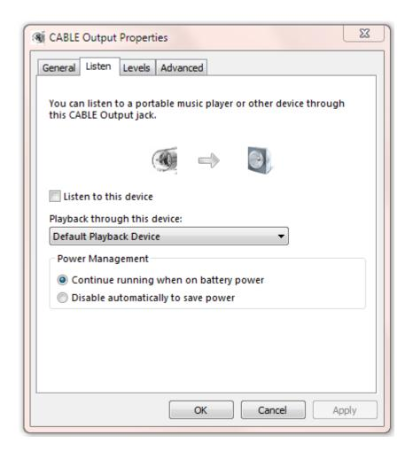
Check the "Listen to this device" box and Apply. You should hear audio from SDR# through the speaker. Leave it on for now during the testing. You might want to turn it off again after it is all working.
