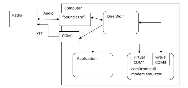
Special software tricks both Dire Wolf and the packet radio application into thinking they are using a pair of physical serial ports connected to each other.
