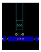
Select it by using the  $\leftarrow$  and  $\rightarrow$  keys. Press the 'm" key to unmute it. The "MM" should change to "00."
