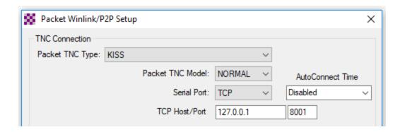
Be sure model is set to NORMAL. ACKMODE will cause an error.
